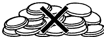
Example of stacked and jumbled batteries
